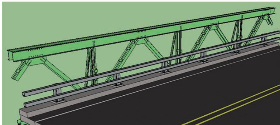
Approximation: ODOT Two-Tube Curb-Mounted Railing (Option 2)
