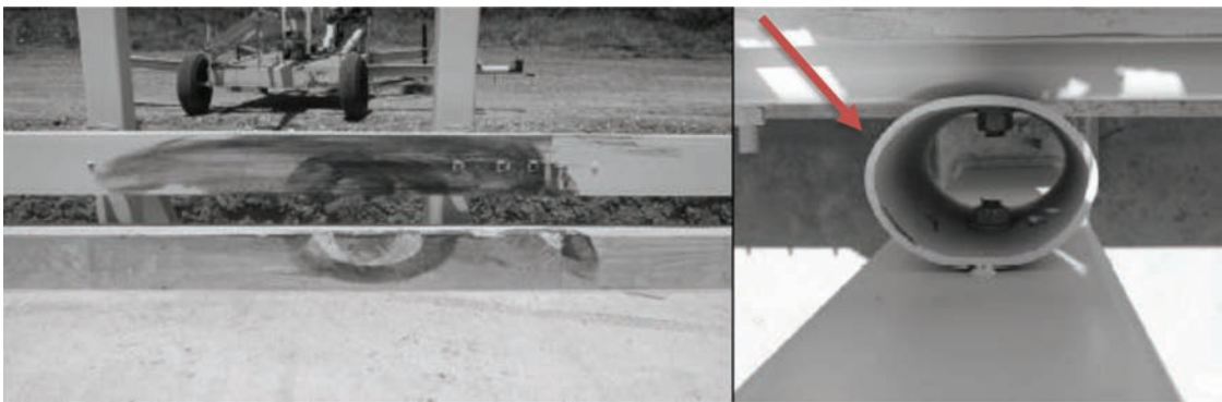
Figure 2.6 Test setup of the Roy B. Inks railing after crash testing (Buth et al., 2004).
