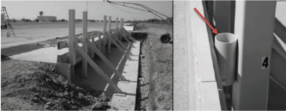
Figure 2.5 Test setup of the Roy B. Inks railing before crash testing (Buth et al., 2004).
