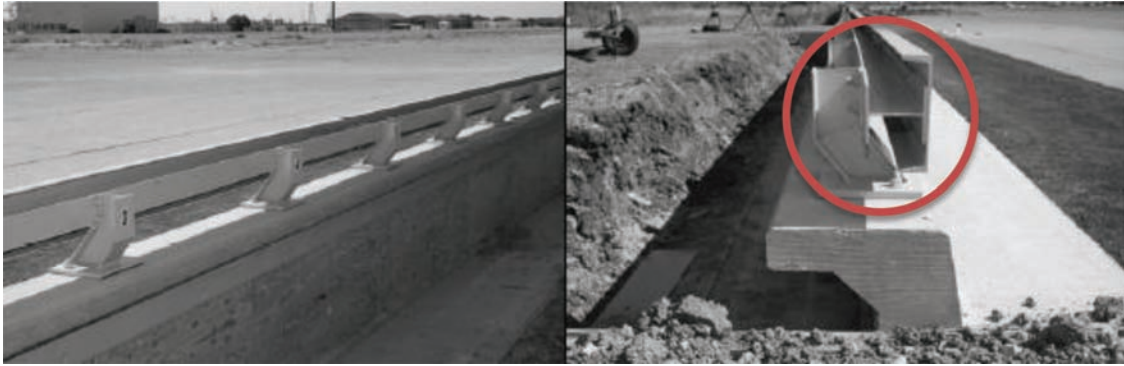
Figure 2.8 Test setup of the U.S. 281 railing before crash testing (Buth et al., 2004).
