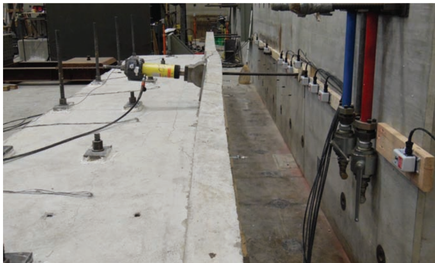
Figure 4.49 Deflected shape at failure (Specimen 2L).
