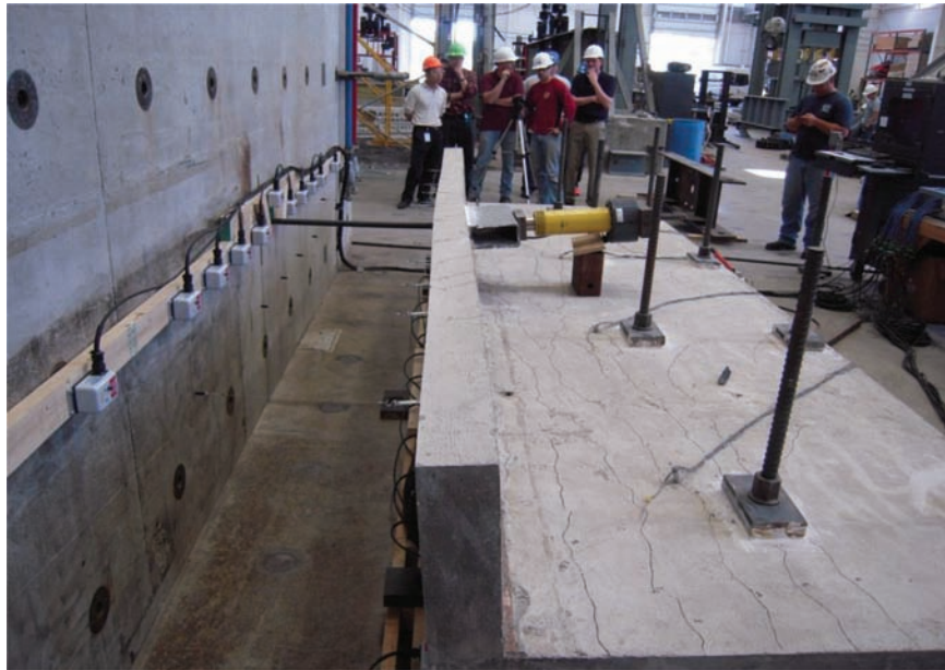
Figure 4.34 Deflected shape at 26.8 kip (Specimen 1).
