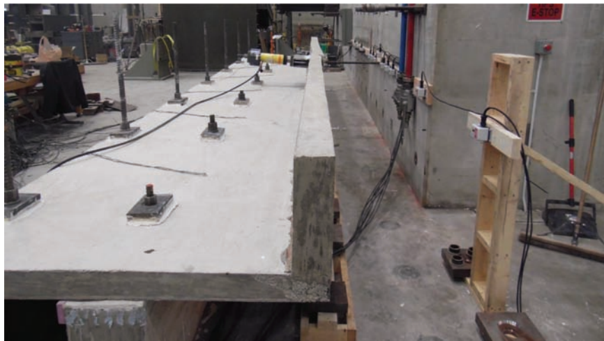
Figure 4.44 Deflected shape at failure (Specimen 1L).
