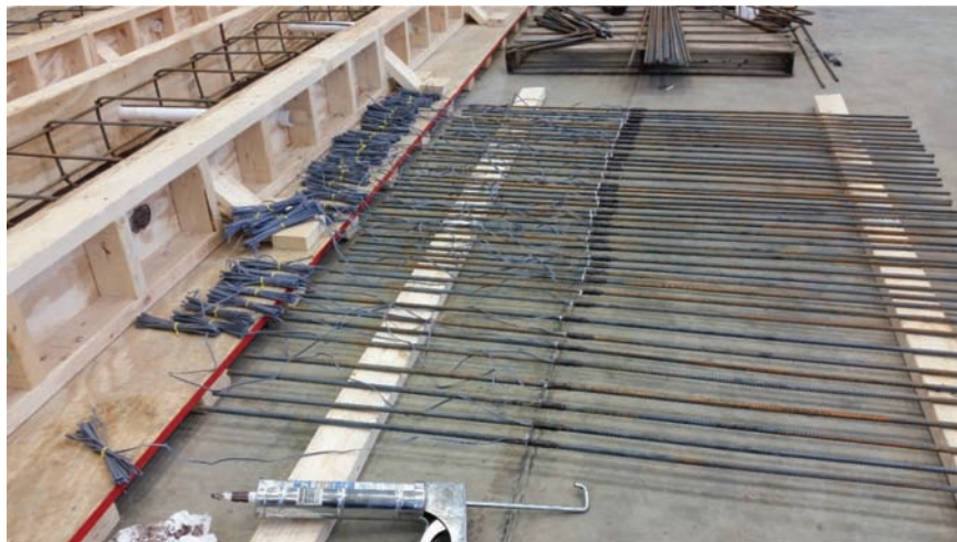
Figure 4.27 Completed strain gages on transverse bars.
