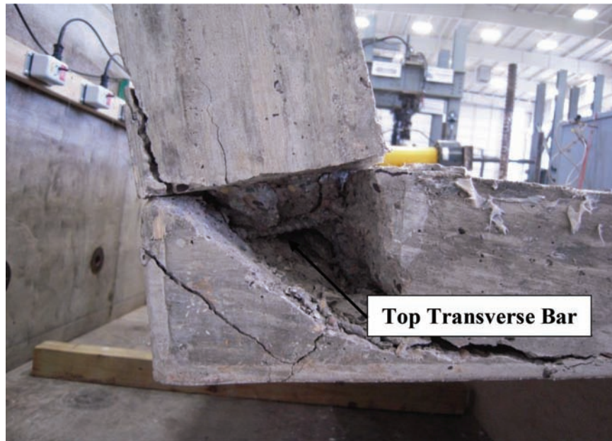
Figure 4.40 Diagonal tension failure (Specimen 2).
