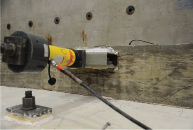
Figure 6.4 Punching shear failure (Specimen 1L).
