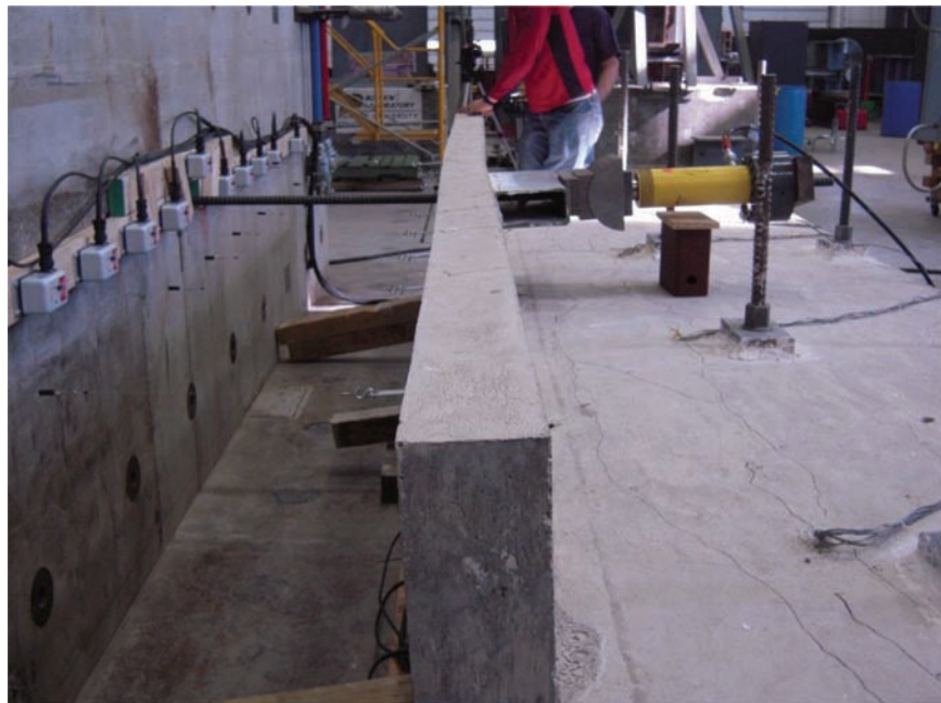
Figure 4.39 Deflected shape at 21.5 kip (Specimen 2).
