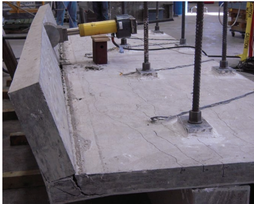
Figure 4.41 Deflected shape after post-peak reloading (Specimen 2).
