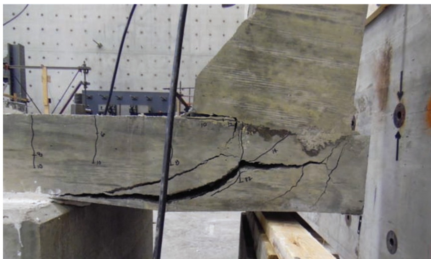
Figure 5.23 Strip Specimen 2 failure plane at 14 kip.
