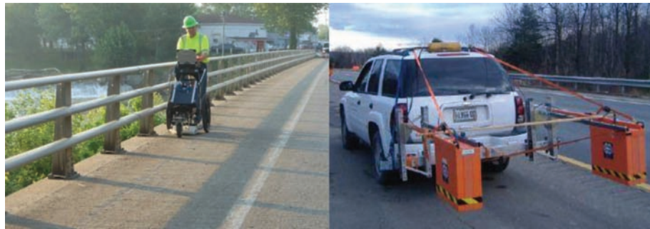
Figure A.8 Ground-coupled GPR system used by INDOT (left). Air-launched horn GPR system on vehicle (right). (Right photograph courtesy of Infrasense, Inc. (Maser et al., 2012).)
