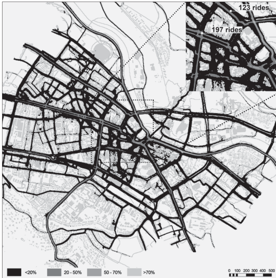
FIG. 2 DENSITY OF RIDES: LAYER ALLROUTES: LAYER REPRESENTED OVER A GRID SUBSTRATE WITH ALL CALCULATED ROUTES OF VARIOUS DRIVERS IN EACH OF THE GRID FIELDS
