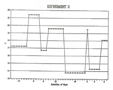
From the surrvey of experiment conditions results, that time of utilization of the evaporation cooling equipment was during experiment No 2. 162 h only (=9.1% of it's total time). The time of utilization was dependent on the weather and activity boundary of equipment (over 24°C).
