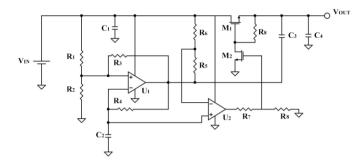
Fig. 9. Simplified schematic of the boost DC/DC converter.
