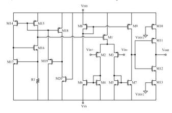
Fig. 6. Designed LV-LP OTA used for the comparator.
