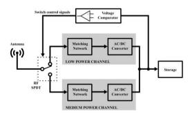
Fig. 2. Simplified scheme of the conceived architecture.
