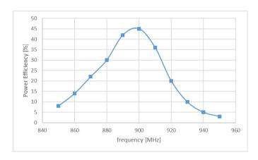
Fig. 11. Conversion efficiency for the medium power channel at 10 dBm input power
