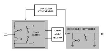
Fig. 4. Block scheme of the integrated version of the harvester.
