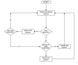
Fig. 5. Flow chart related to the indoor/outdoor positioning process.
