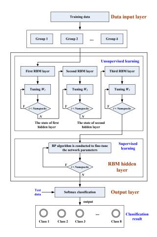
Figure 2. The flowchart of RSRDRBM algorithm.
