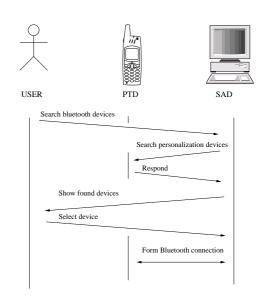
Fig. 6. Forming SAD-PTD Bluetooth connection
