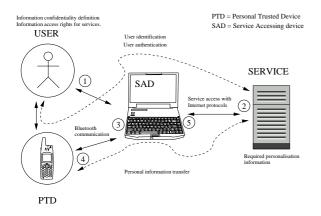
Fig. 4. General service access architecture and operations
