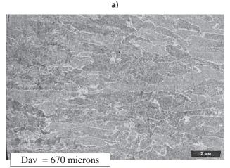
b) Figure 1 Macrostructure of cast metal
