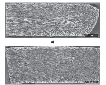
Figure 4 Dendritic structure of the strip after controlled rolling: a) no modifiers added; b) modified by AKCeZh 2,3 kg/t
