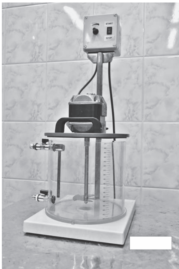
Figure 2 View of a mechanical particles stirrer together with the water tank
