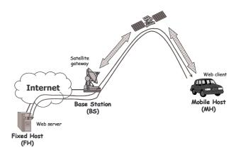
Fig. 1. A mobile host accesses an Internet fixed host through a satellite link.
