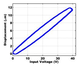
Fig. 9. Experimental result of hysteresis loop in open-loop without compensation
