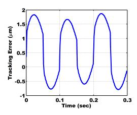
Fig. 13. Experimental result of tracking error in open-loop without compensation
