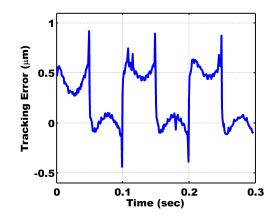
Fig. 14. Experimental result of tracking error in open-loop with feed-forward compensator
