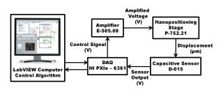
Fig. 2. Block diagram of experimental loop
