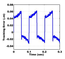
Fig. 15. Experimental result of tracking error in closedloop with full-order  $H_{\infty}$  feedback controller in the presence of feed-forward compensator
