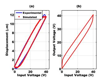
Fig. 5. (a) Experimental and simulated hysteresis loops with a triangle input voltage of amplitude 40 V and frequency of 10 Hz (b) Output response of the inverse estimated Prandtl-Ishlinskii hysteresis model
