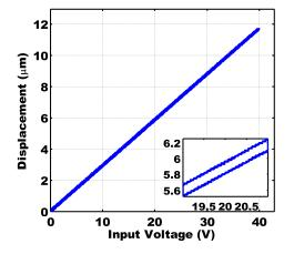
Fig. 12. Experimental result of hysteresis loop in closedloop with fixed-order  $H_{\infty}$  feedback controller (HIFOO) in the presence of feed-forward compensator
