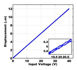
Fig. 11. Experimental result of hysteresis loop in closedloop with full-order  $H_{\infty}$  feedback controller in the presence of feed-forward compensator
