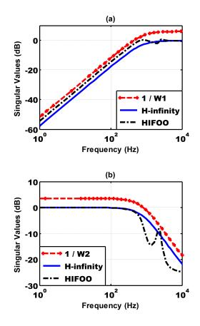
Fig. 8. (a) Magnitude response of output sensitivity function **S** and weighting function  $1/W_1$  (b) Magnitude response of complimentary sensitivity function **T** and weighting function  $1/W_2$
