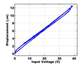
Fig. 10. Experimental result of hysteresis loop in open-loop with feed-forward compensator
