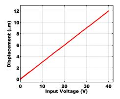
Fig. 6. Simulation result with inverse estimated Prandtl-Ishlinskii hysteresis model as a feed-forward compensator
