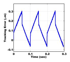
Fig. 16. Experimental result of tracking error in closedloop with fixed-order  $H_{\infty}$  feedback controller (HIFOO) in the presence of feed-forward compensator
