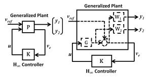
Fig. 7. Generalized plant (P) with controller (K) in  $H_{\infty}$  framework
