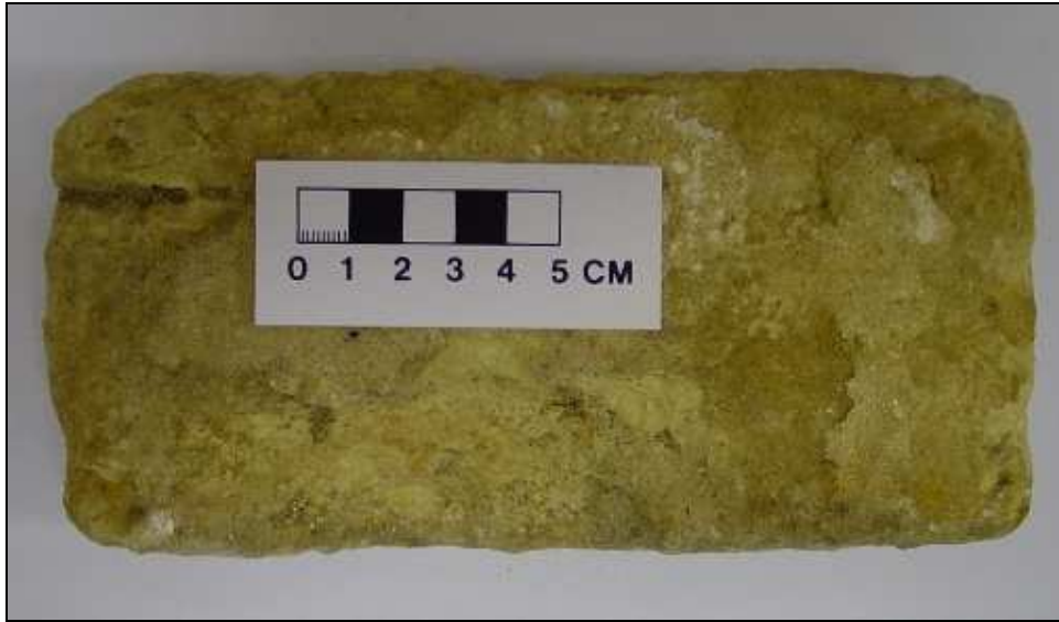
Fig. 2.5: An example of a 'Flemish' type brick.
