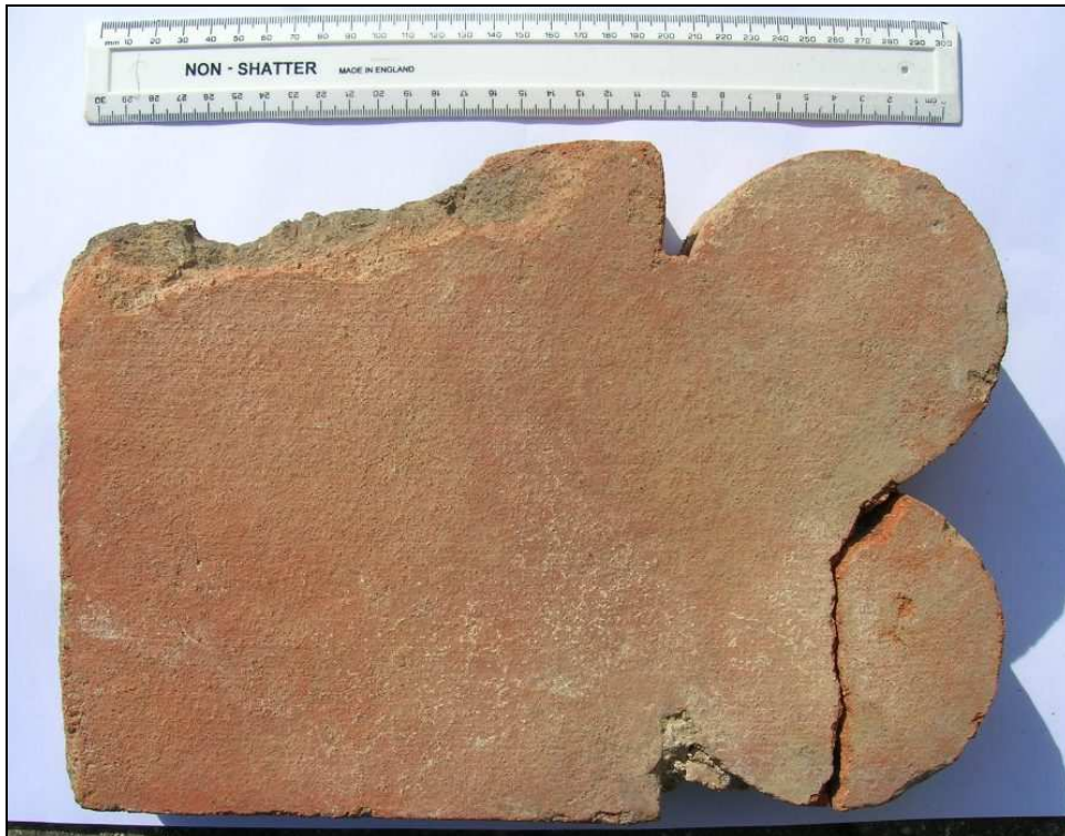
Fig. 2.2: Example of a moulded brick form used at Coggeshall Abbey (Pat Ryan, 2007).
