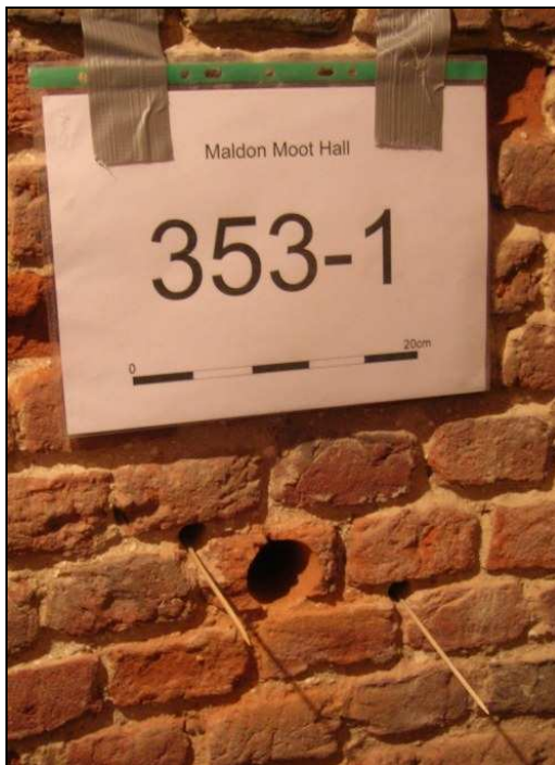
Fig. 4.4: Images illustrating the different stages in collecting a sample. The top image shows the brick selected for sampling being sampled with the electric core drill. The bottom left image shows the resulting hole after the core had been removed and the smaller holes in the mortar into which dose capsules have been inserted (the sticks to which the capsules are attached protrude from the wall face). The bottom right image shows the repair work done to the brick (circled) after sampling had been completed (the protruding parts of the dose capsule sticks were snapped off to prevent further disturbance to the capsules). The scale in the images is 20 cm in length.
