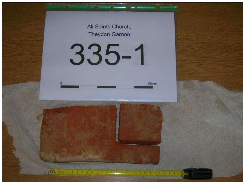
Fig. 3.107: The brick that was removed from the wall for sampling. The image shows the rear portion that was removed from the main brick. A second portion was also removed by means of a diamond tipped hand saw in an attempt to derive the water content for this brick. The scale is 20 cm in length.
