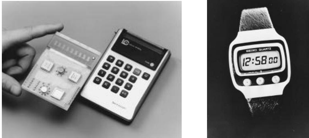
Figure 11. (a) The world's first commercially available LC product, a pocket calculator, developed by Tomio Wada, Tadashi Sasaki and their team at Sharp in 1973 reprinted from reference [124] © 2002 IEEE. (b) Seiko Watch Company introduces their first digital watch with a twisted nematic LC display to the commercial market reprinted from reference [124]
