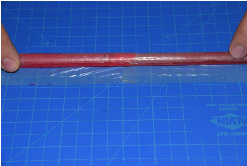
Figure 4.5 Rolling of the latex on the dowel
