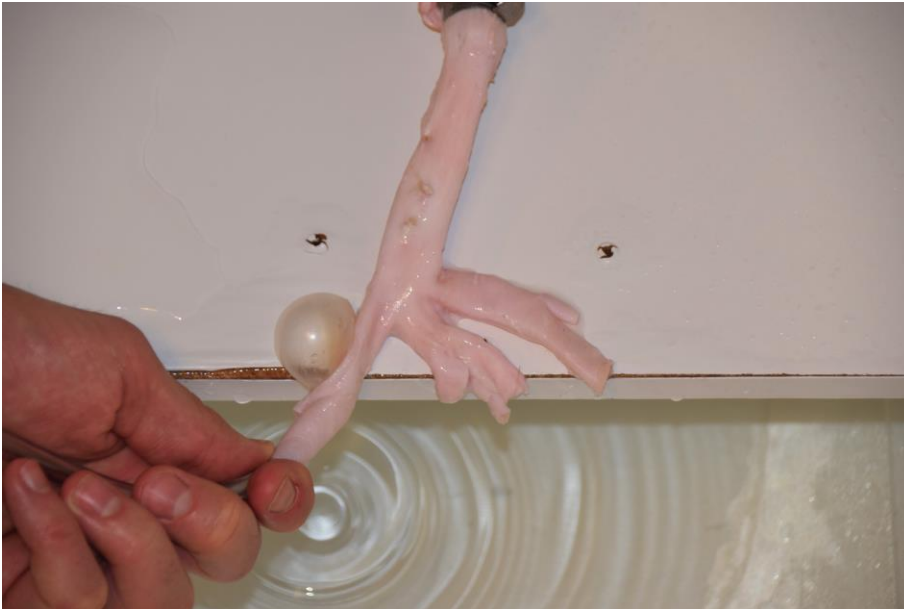
Figure 4.20 Porcine aorta with iliac defect occlusion testing
