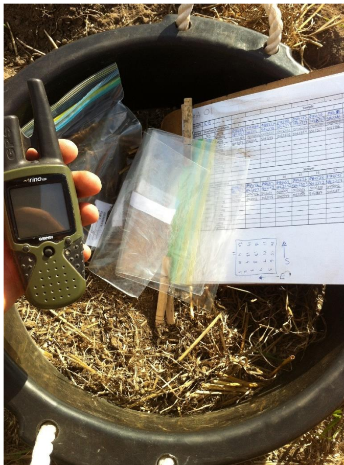
Figure 2.5 Improved plastic sampling frame, GPS unit, resealable grain sample bags, and sample point data sheet in use during field work. Sampling frames were built by removing the bottom of generic, plastic grain buckets and were used for collecting waste agricultural grain from known area units in harvested agricultural fields at Manitoulin Island, Ontario, Canada in autumn 2011 and 2012.
