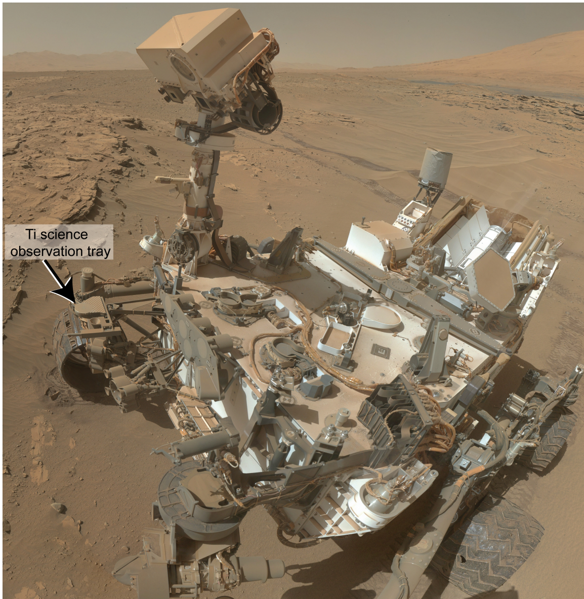
Figure 4-S1. Location of the Ti Science Observation Tray (o-tray) on Curiosity . The MAHLI mosaic [after JPL Photojournal http://www.nasa.gov/jpl/msl/pia18390 ] shows the o-tray mounted on the right-front of the rover, coated with dull red-brown dust, which covers most of the surfaces of the rover. These images were acquired on Sol 613, 42 sols
