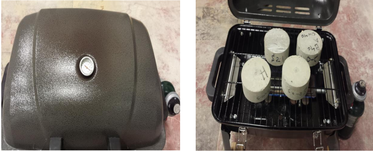
Figure 5-3: Heating chamber setup.
