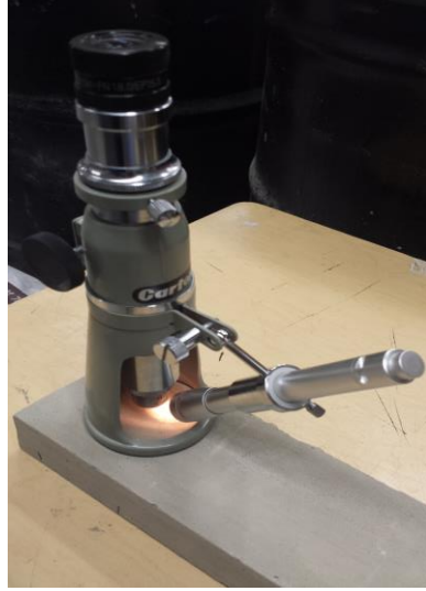
Figure 3-2: Crack monitoring optical microscope.
