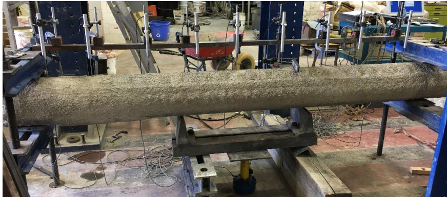
Figure 5.4 Bending test setup on extracted pile
