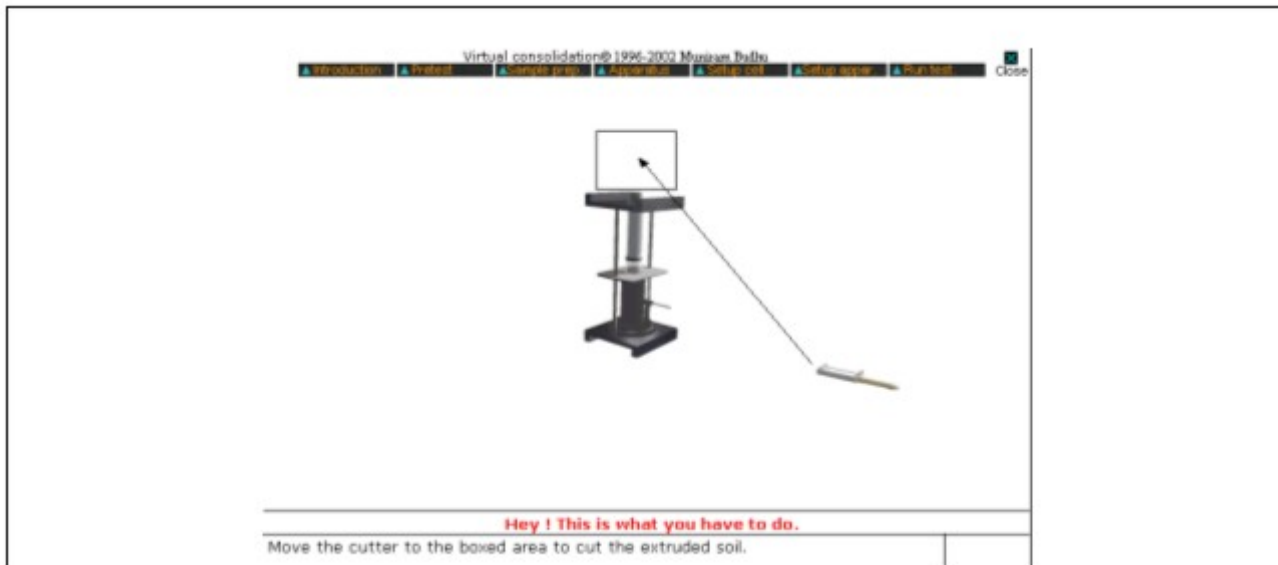
Figure 6: The user is prompted to move a cutter to cut out part of a soil sample during sample preparation.
