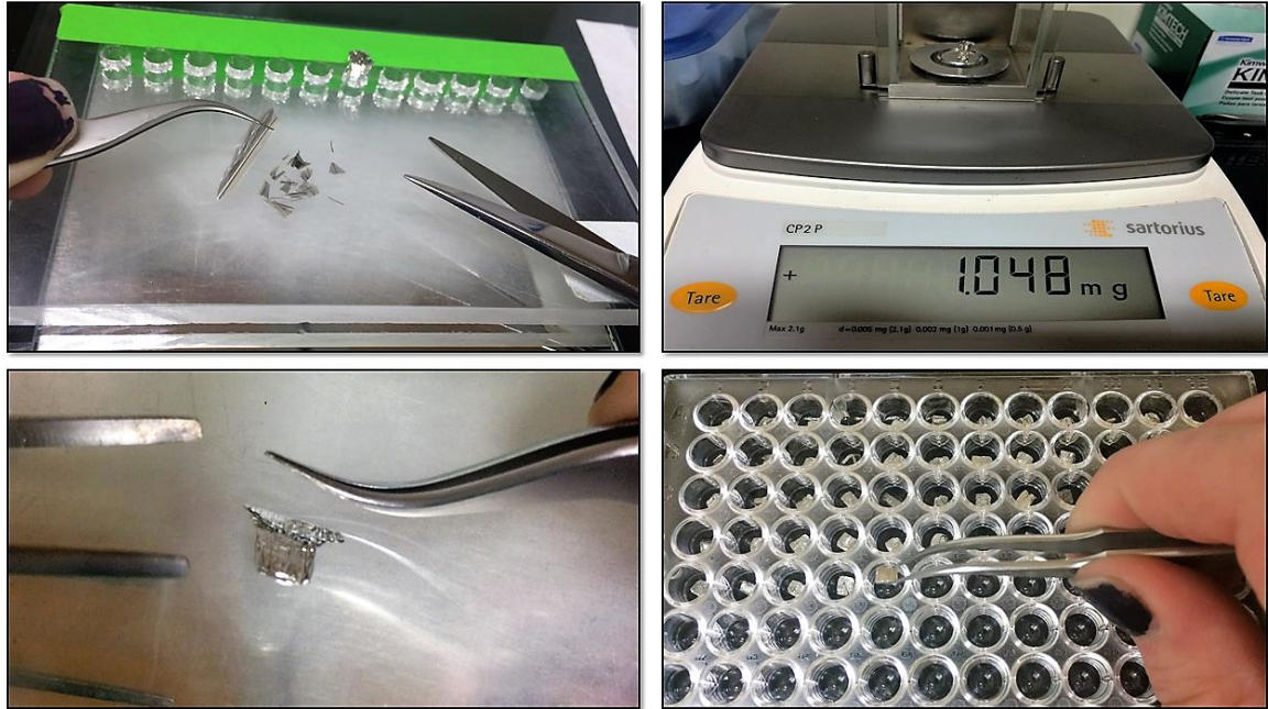
Figure 8. Photos of sample preparation procedures. On the top left feathers are being cut and placed in a capsule; on the top right feather pieces are weighed in a capsule; on the bottom left the capsule containing the feather pieces is encapsulated into a small ball; and on the bottom right finished samples are placed into a 96 well plate. (E. Moffitt, personal photographs, February, 2015).
