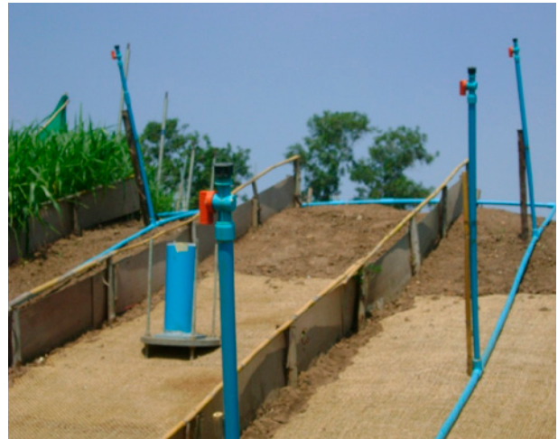
Fig. 9. Set up artificial rainfall
