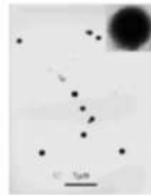
Fig. 7. TEM image of the nanoparticles prepared at pH 5.0.
