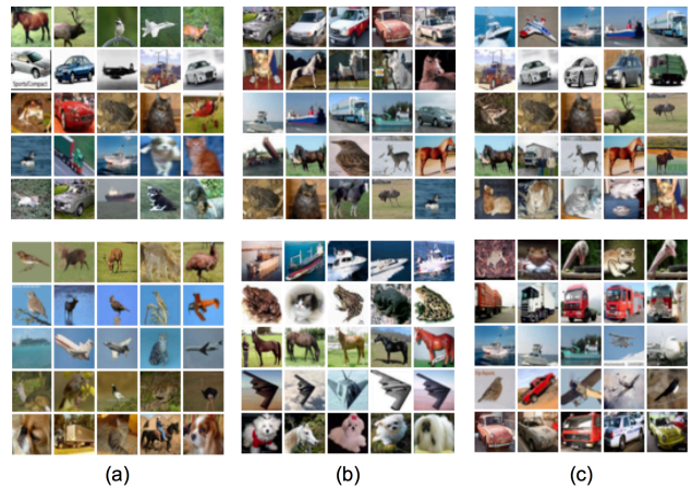
Figure 7. CIFAR-10 clusters used as pseudo-labels (Each row in an represent a different class). All clusters were generated on raw CIFAR-10 images by applying k-means with initial centroids randomly selected. For images in top row k = 10 and for the bottom row k = 100 . Different algorithms were used for dimensionality reduction. (a) 3D color histogram with 8, 8, 8 bins for red, green and blue (512 dimensions). (b) HOG is with cell size 16 \times 16 , 16 gradient bins, stride of 16 (64 dimensions). (c) HOG is with cell size 8 \times 8 , 16 gradient bins, stride of 8 (256 dimensions).
