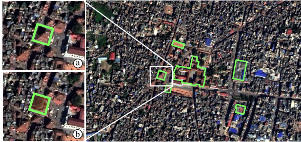
Figure 3. Nepal earthquake, 2015. Compositing vector objects to quickly identify buildings of interest and make a preliminary damage assessment. (a) Close-up on a building, showing imagery captured before the disaster. (b) Compositing post-event imagery inside these buildings only.
