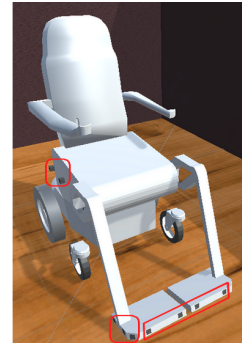
Fig. 3: Virtual Wheelchair. Red frames indicate virtual sensor positions.
