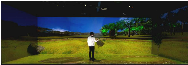
Fig. 1: Immersia is one of the largest VR research platforms in the world. It is composed of 4 large screens on which images are projected for a total volume of approximately 90m^3 . The 3D rendering is achieved by using active stereoscopic method associated with shutter glasses. 16 infrared cameras track the moving objects on the platform.
