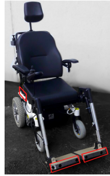
Fig. 2: Real Wheelchair. Red frames indicate ultrasonic sensor positions.
