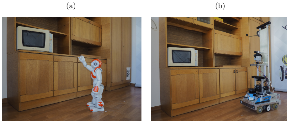
Figure 15: Robots performing hazard detection: (a) NAO humanoid robot, (b) six-wheel Elektron robot
