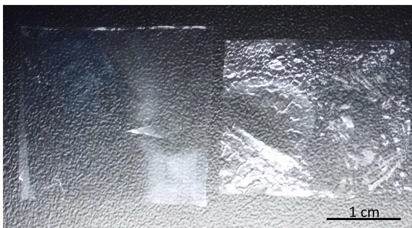
Figure 44: Pictures of spider silk films produced using the film applicator before (left) and after (right) the autoclave post-treatment.
