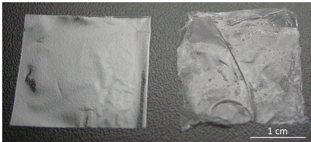
Figure 41: Pictures of spider silk films produced using the film applicator before (left) and after (right) the phosphate ions post-treatment.
