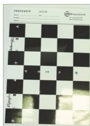
Figure 2: Plastic foil A5 22/5B from mtv-messtechnik (Cologne, Germany) used as substrate to cast spider silk films
