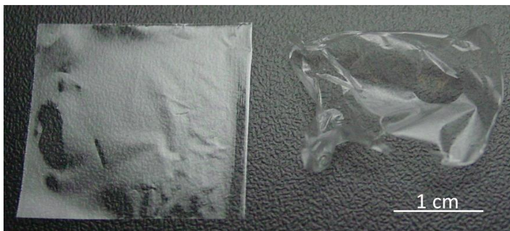
Figure 42: Pictures of spider silk films produced using the film applicator before (left) and after (right) the ethanol post-treatment.
