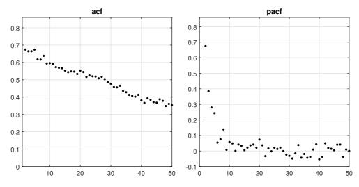
Figure 3.6: Sample (partial) autocorrelation function of 1000 observations from the ARMA(1,1) process given in (3.5.2).
