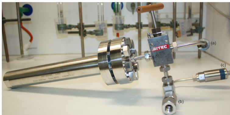
Figure 3.1-1. Autoclave used for ammonothermal reactions, constructed by engineers at university of Erlangen. Insets are described in the text. 28
