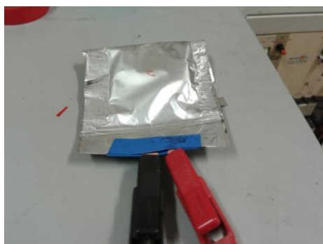
Figure 8.1 - Example of pouch cell assembled for ex-situ NMR measurements (on the left) and voltage profile of NB0D0 and NB15D5 samples: red circles indicate the voltage to whom electrodes have been recuperated.
