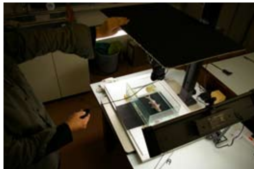
Photography with a black background. A black board is placed between the white board and the aquarium base. In order to avoid reflection of roof barre and lamp in the glass of the aquarium base, it is necessary to hold a large black board above the camera.
