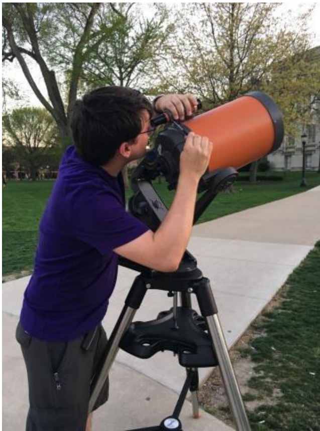
Dominic Ludovici collimating a telescope.
