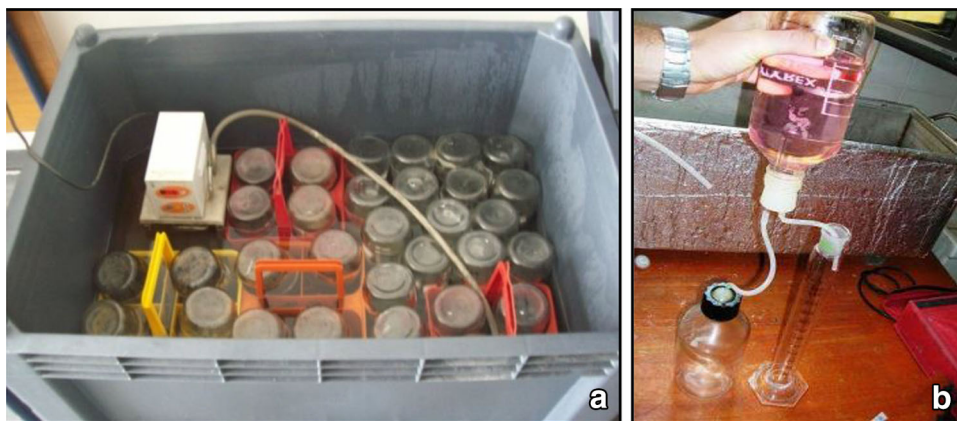
Fig. 3 Lab tests experimental equipment. Mesophilic water bath containing the BMP bottles (a) and manual measurement of the biogas produces through water displacement (b)
