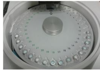
Figure 5. Lubricants ready to be tested in the DSC/TGA test
