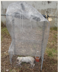
Figure 1: A modified version of the Malaise trap used to capture insects attracted to a carrion. A glass bottle was coupled to the upper net to capture flying specimens, and a plastic container was placed at the bottom to capture crawling insects.
