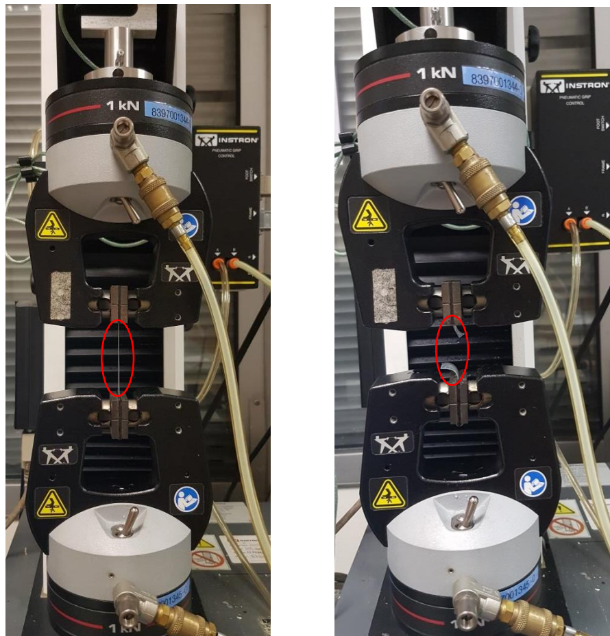
Figure 4- 1. Mechanical Testing with Instron Machine. Specimens (i.e. silk films and PolyJet Materials; circled in red) were clamped between the pneumatic clamps and
