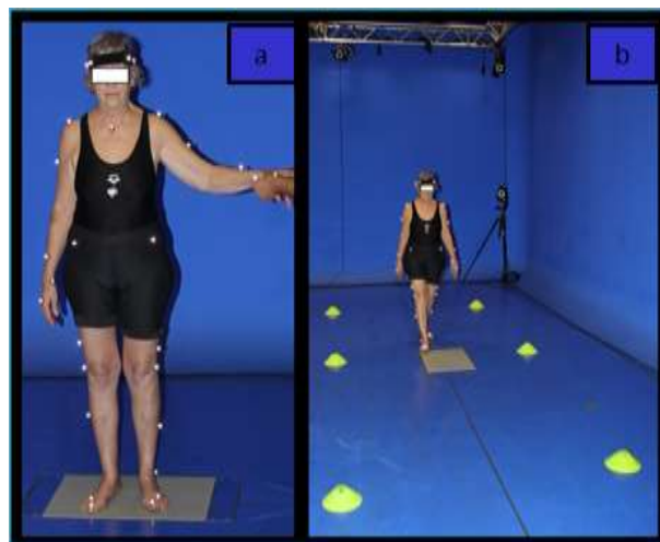
Figure 25. The spherical reflective markers that make up the three-dimensional model in use (25a) and the 7-meter walkway (25b).
