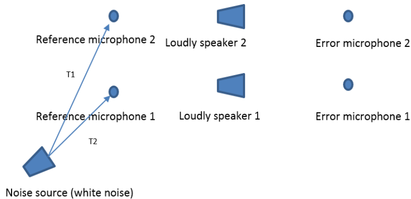
Figure 3-10 CR 2x2x2 ANC system position diagram
