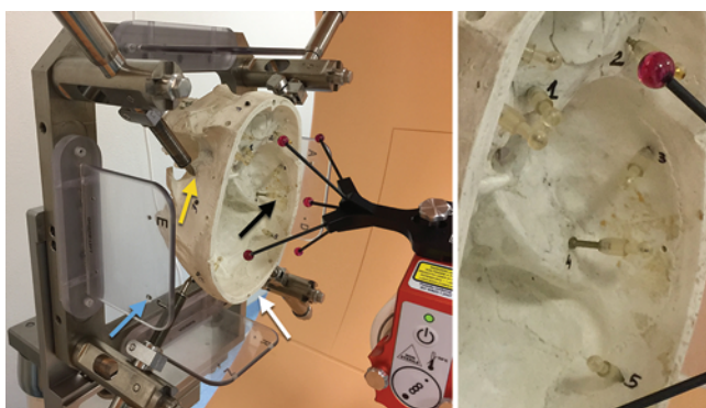
FIG. 3. Left: Photograph of the phantom study setup showing the attachment of the plastic skull to the Talairach frame, the FMs, and the localizers. The plastic skull ( white arrow ) is attached to the pillars of the Talairach frame by means of 4 conical pins ( yellow arrow ). Ten FMs with removable targets ( black arrow ) are fixed to the internal skull. The localizers ( blue arrow ) for bidimensional x-ray registration are attached to the base of the frame. Right: Close-up view of the plastic skull and removable targets.
