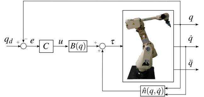
Fig. 3. The motion control scheme with the inverse dynamics-based feedback linearization applied to the robot system.
