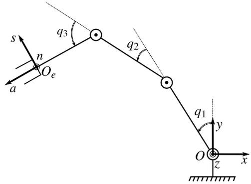
Fig. 2. A schematic planar view of the robot manipulator with the joint variables.
