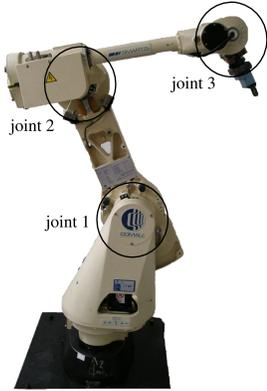
Fig. 1. The COMAU SMART3-S2 anthropomorphic industrial robot manipulator used for the tests with the joints numeration.
