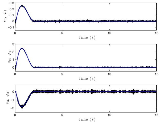
Fig. 6. From the top: the sliding variable  $s_i$  (solid black line) and the transient function  $\varphi_i$  (solid blue line) for joint 1,2 and 3, respectively (simulation results).
