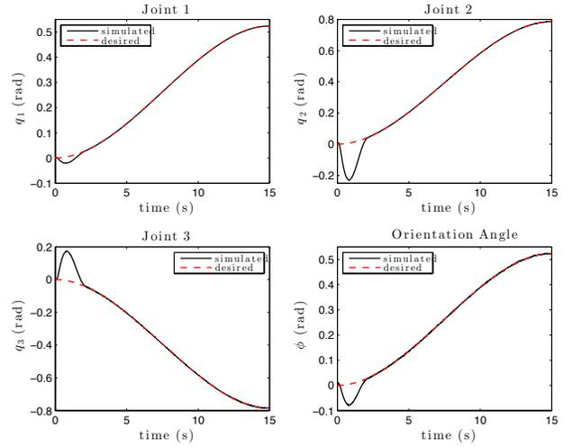
Fig. 4. Angular position of joints and end-effector orientation angle  $\phi$  (simulation results). From the top on the left: the desired trajectory (dotted red line) and the real one (solid black line) for each joint.
