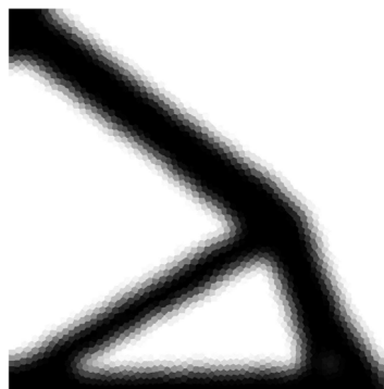
Fig. 13. Compressible elasticity. Example 2: square cantilever. Optimal topology computed with the proposed VEM-based formulation on an unstructured mesh with 2^5 elements along the thickness of the cantilever and filter radius r_{\min} = 3.0d_m \approx 1.5/2^5 .
