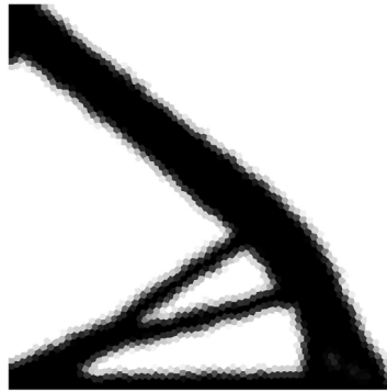
Fig. 12. Compressible elasticity. Example 2: square cantilever. Optimal topology computed with the proposed VEM-based formulation on an unstructured mesh with 2^6 elements along the thickness of the cantilever and filter radius r_{\min} = 1.5d_m \approx 1.5/2^6 .
