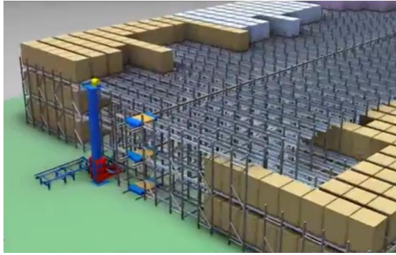
Figure 1. Illustration of a shuttle-based compact storage system (source: Total Solution Provider Group).
