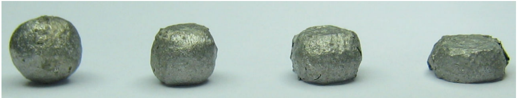
Fig. 3. Compression phases of a single APM foam element.
