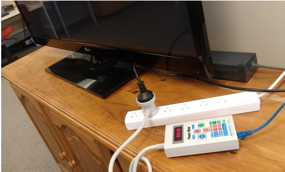
Figure 3.11. Example of measuring the power consumption of a TV using Power-Mate 10AHD Serial.
