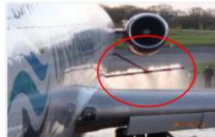
Boeing 727 jet-based aerial dispersant system
