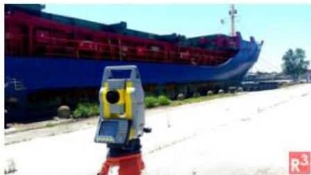
TOTAL STATION SURVEY
