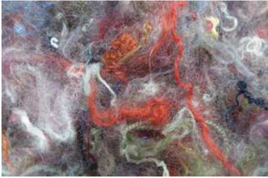
Reclaimed fibres from post-consumer textile waste and re-spun into new yarn (source: Texperium)
