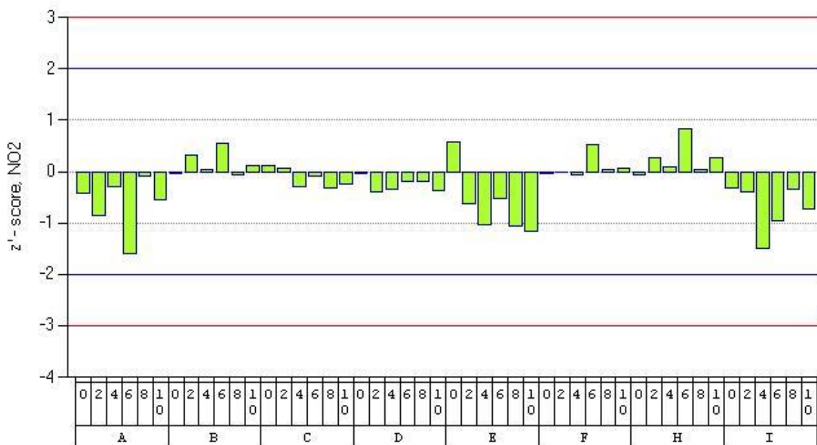
Figure 5: Z'-score evaluations of NO 2 measurements
