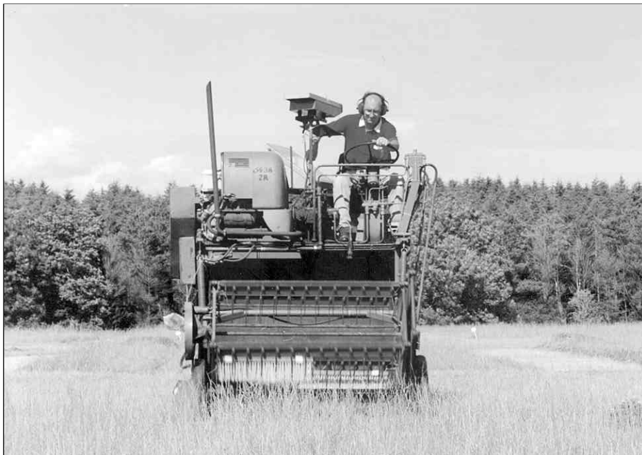
Plate 3. Harvesting of grass plots using the Haldrup plot cutter.
